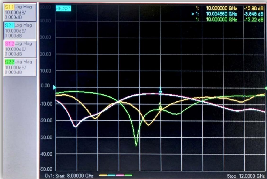
Figure 5.7 Measured S-parameters of ON-state of SPDT switch
