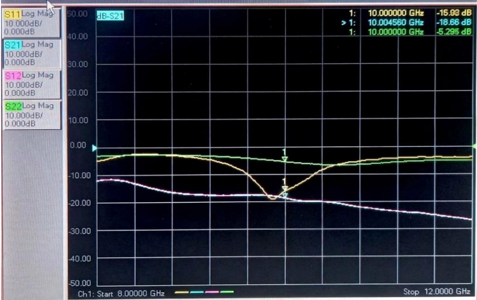
Figure 5.8 Measured S-parameters of OFF-state of SPDT switch
