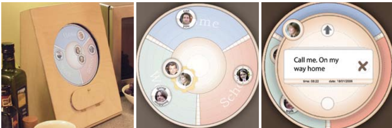
← The Whereabouts Clock: the lefthand image shows the clock in its case; the middle image is a close-up of its interface; and the righthand image shows what happens when you touch on a text message.
