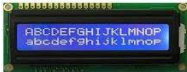
Figure 24: LCD (16*2) for display of results
