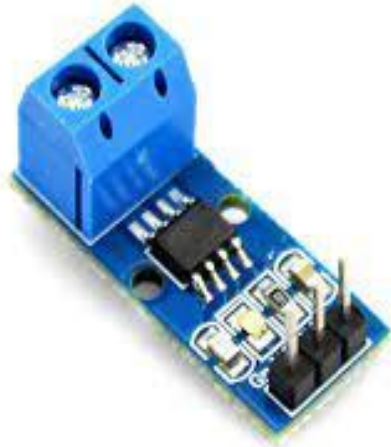
Figure 23: ACS 712 for Current measurement
