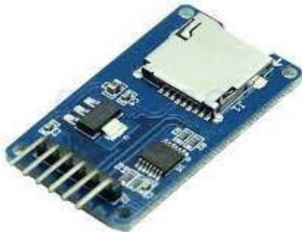
Figure 26: SD Card Module to store results
