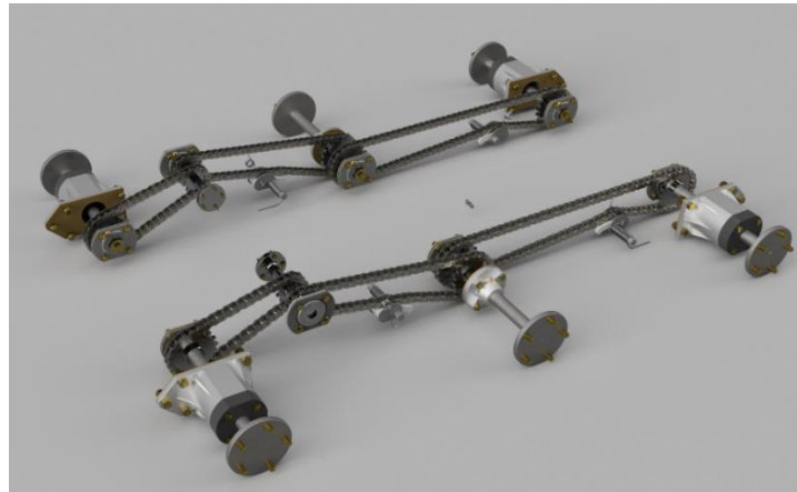
Figure 14: Chain Sprocket Mechanism of Argo
