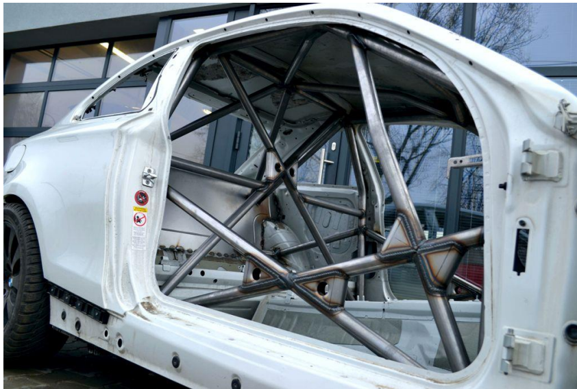
Figure 23: At typical Roll Cage fitted inside a vehicle
