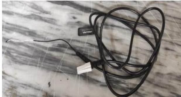
Figure 12. Vernier Surface temperature sensor used in testing; the white tip of the sensor was introduced to the testing area.
