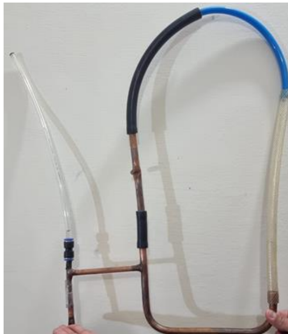
Figure 8. Constructed basic configuration hand model of fluidyne.
