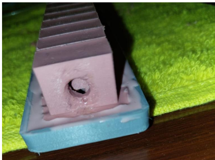
Figure 23. Hole made for connecting the air source
