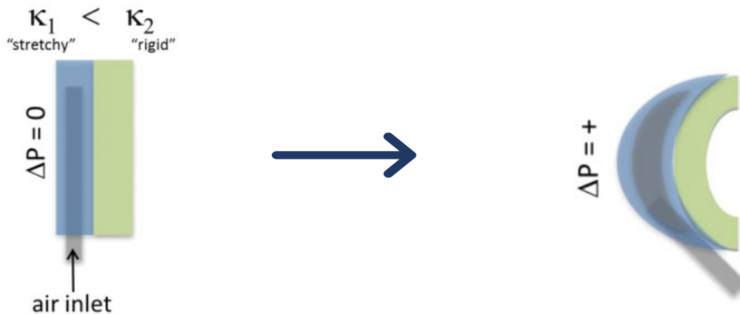
Figure 5. Working Principle (Bending motion displayed)
