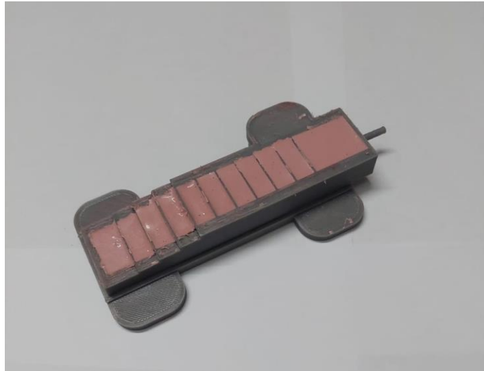
Figure 30. Top part of actuator curing
