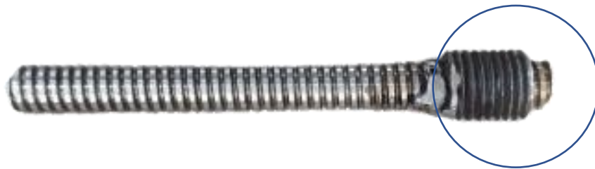
Figure 32 Additional Thread on the Power Screw
