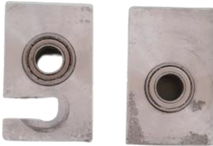
Figure 31 Both Parts of Bearing Housing
