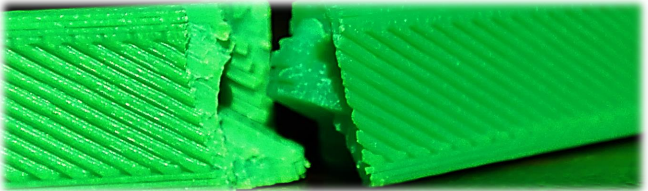
Figure 35: Crack propagation in 45H Sample
