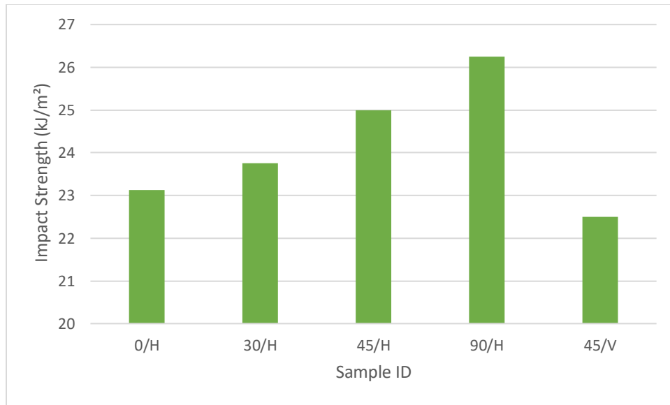
Figure 26: Impact Strength of PLA without heat treatment
