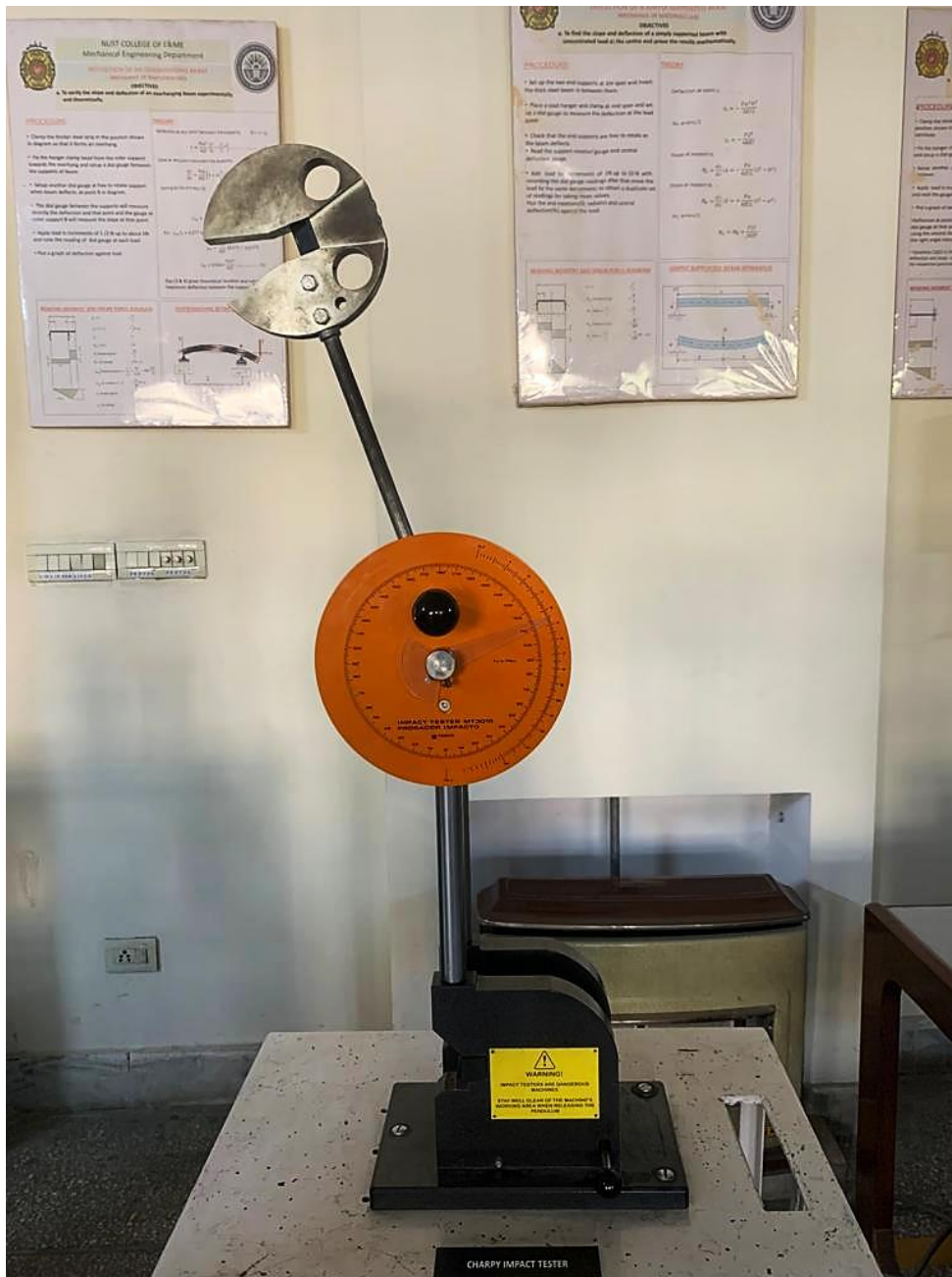
Figure 19: Charpy Impact Test Apparatus used for Impact Testing of the samples
