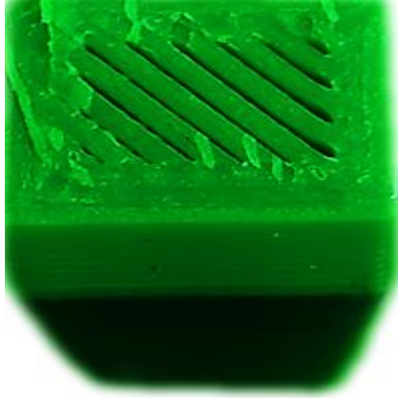
Figure 34: Crack propagation in 45V sample
