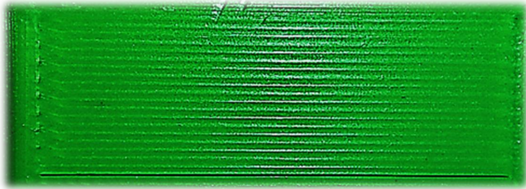
Figure 32: Sample Printed at a raster angle of 0^\circ
