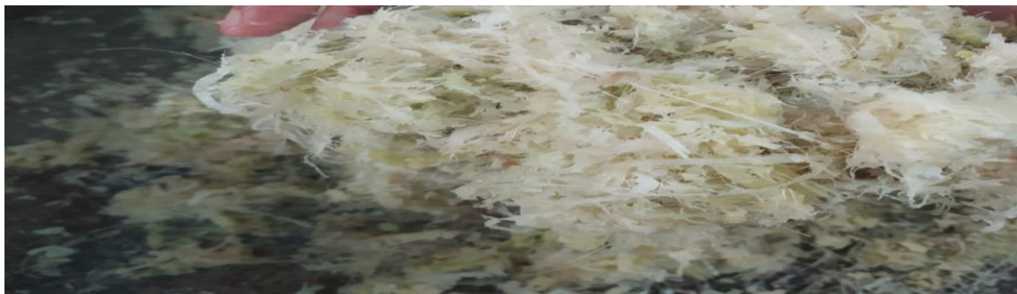
Figure 43. Residue collected during decorticator operation
