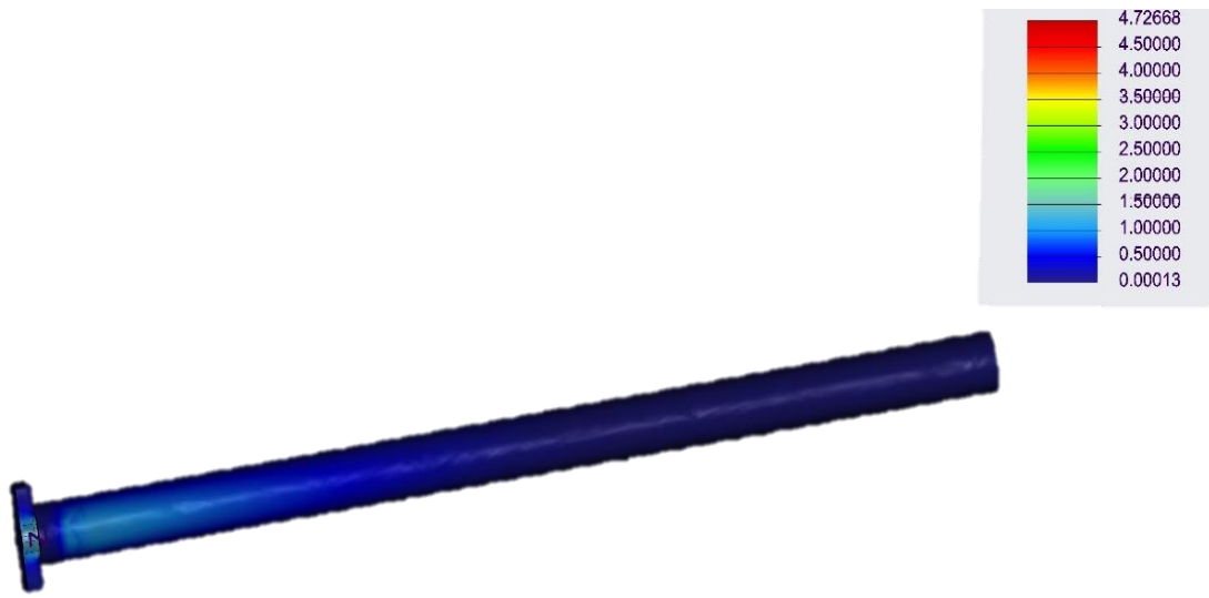
Figure 4-2: Stress for fully extended horizontal manipulator
