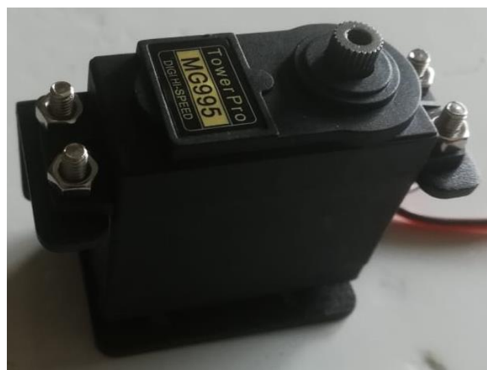
Figure 5-13: Servo motor installed in its bracket
