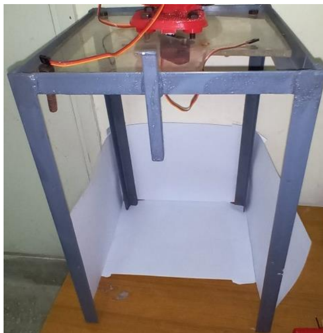
Figure 6-1: Assembled platform and Joint J1
