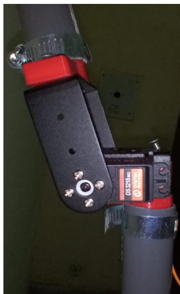
Figure 6-3: Joint J3 fully assembled
