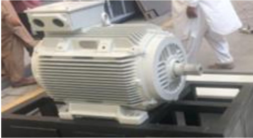
Figure 12: Siemens 45 KW Motor
