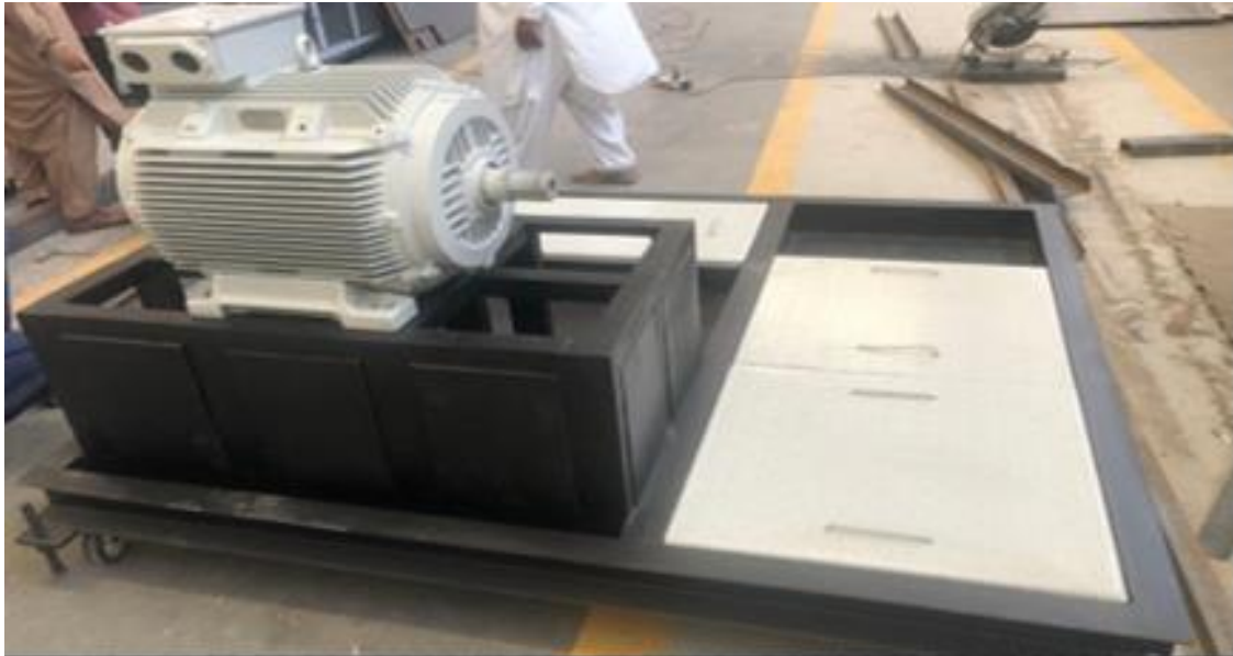
Figure 35:HTB base with motor installed
