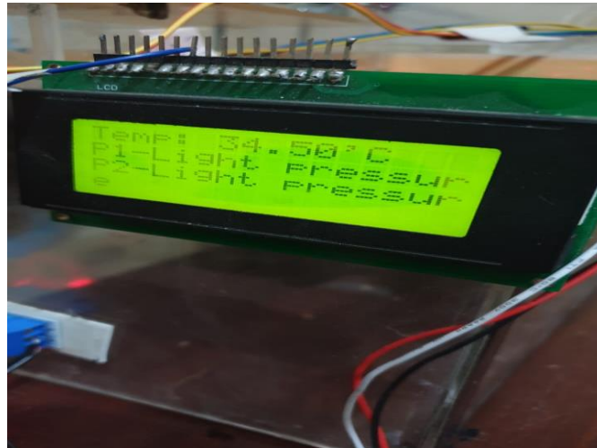
Figure 50 Pressure sensor readings
