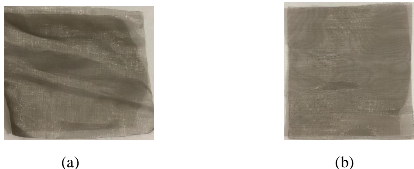
Figure 3. 32 Two different sized sieves mesh (a) 53 microns sieve mesh (b) 63 microns sieve mesh
