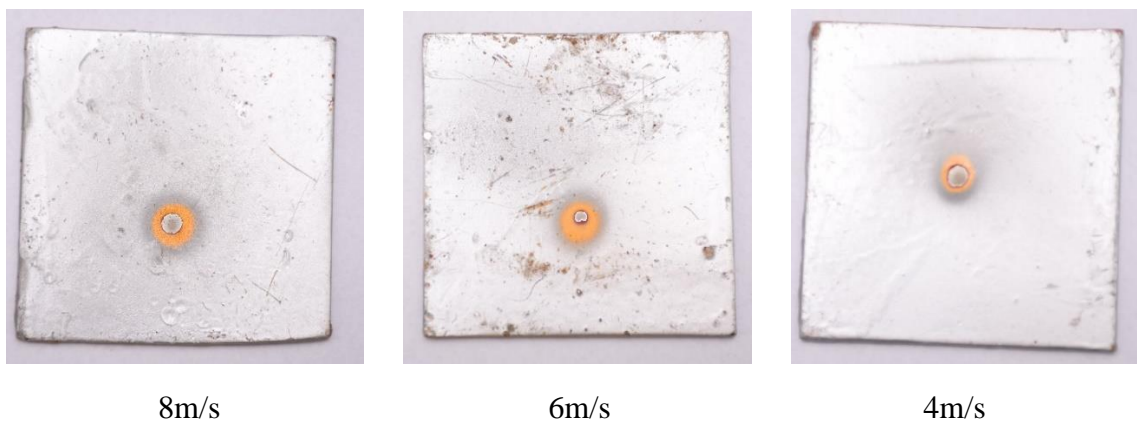
Figure 4. 2 Paint erosion pattern for erosive solid-liquid flow with 90-degrees impact angle
