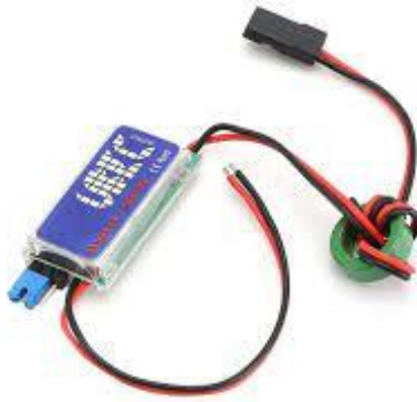
Figure 41 UBEC, a switching regulator
