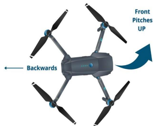
Figure 12 Drone pitching backwards
