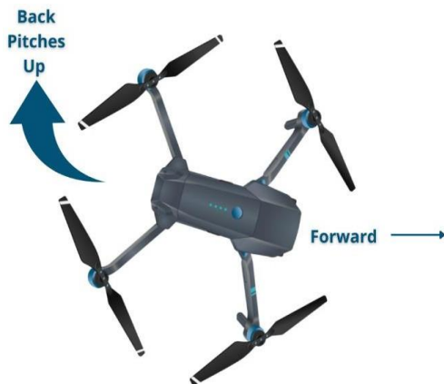
Figure 11 Drone pitching forward
