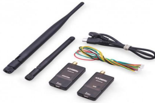
Figure 39 Telemetry kit and its components
