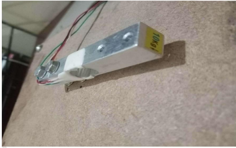
Figure 22 Load Cell position (Testing Phase)
