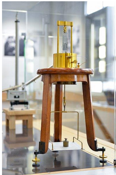
Figure 1 Piezoelectric quartz device that belonged to the Curie Laboratory courtesy of the Curie Museum
