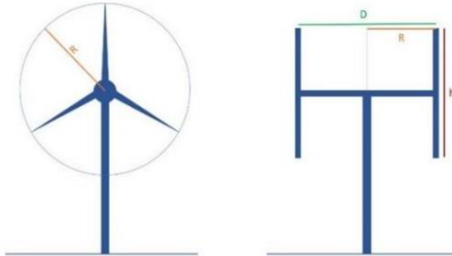
Figure 2 Typical Horizontal (left) and vertical axis turbines (right)
