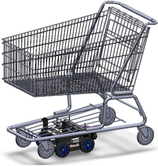
Figure 3-9: Assembly of Power Kit attached to Wheeled Cart
