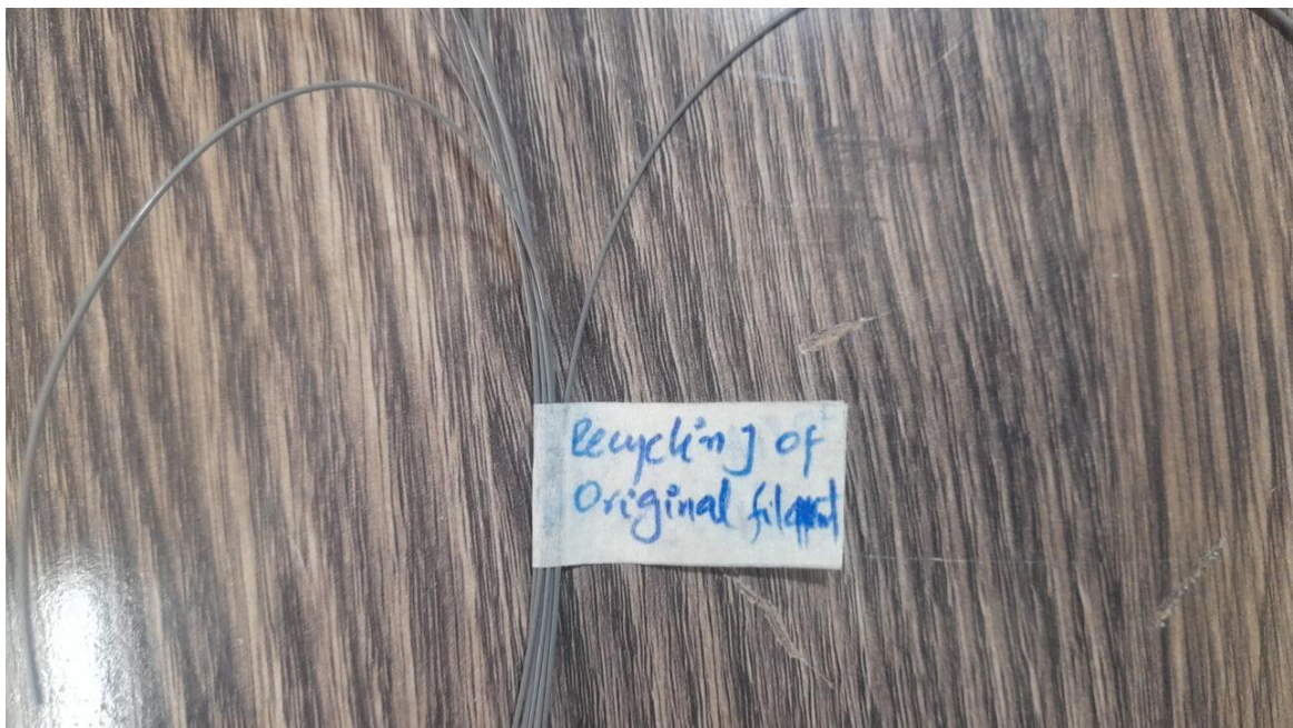
Figure 53: Filament produced from pellets at 180 Degree Celsius
