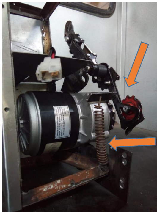
Figure 5.15: Spring loaded idler for proper tension
