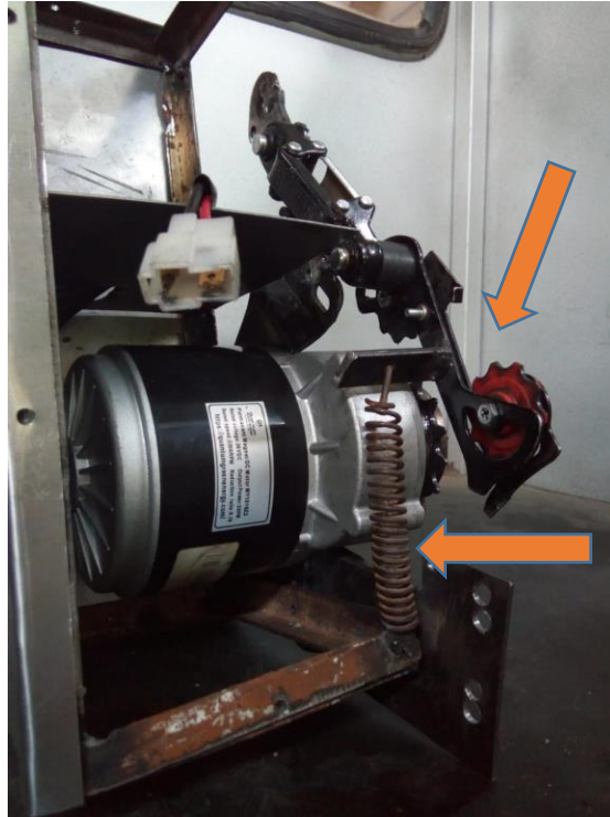
Figure 5.8: Spring loaded idler arm
