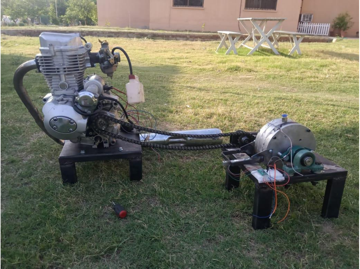
Figure 4-1: Dyno and Engine mounted on the beds.
