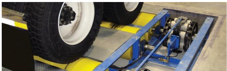
Figure 1-5: Chassis dyno, with eddy current brake visible.
