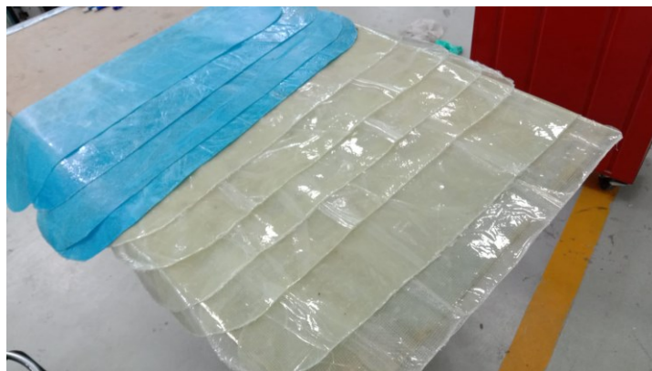
Figure 32: Prepreg sheets ready for layup
