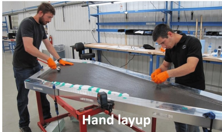
Figure 2: Hand Layup Process for Prepreg Man
