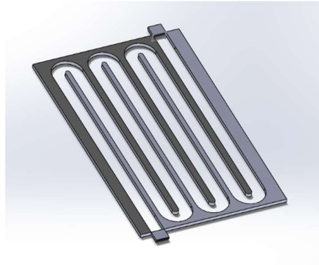
Figure 8.1: Cooling plate initial design
