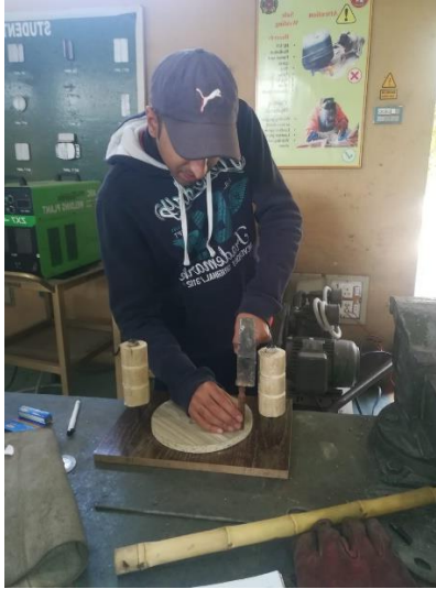
Figure 4.13: Pressing the crank into the crank base.
