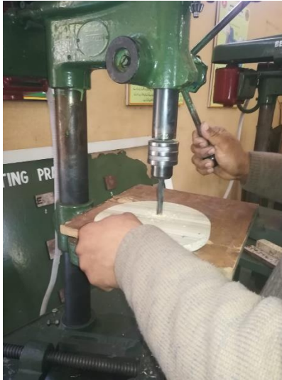
Figure 4.11: Drilling holes into the crank base
