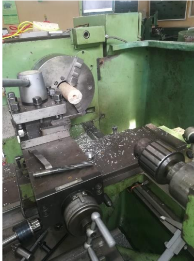
Figure 4.9: Drilling holes in Pulley
