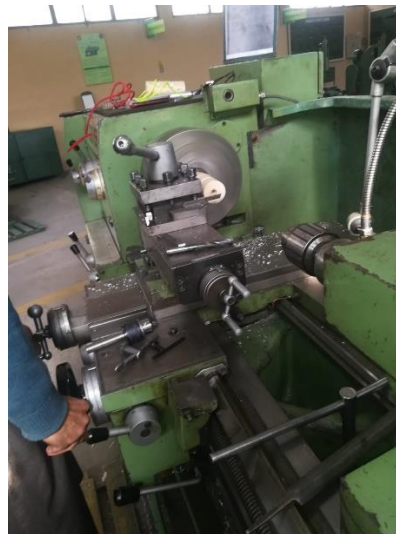
Figure 4.8: Machining the pulley
