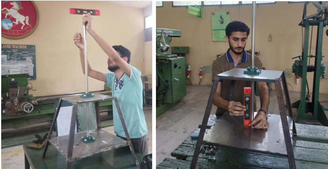
Fig 61. Bubble Level for Shaft and Bearings alignment
