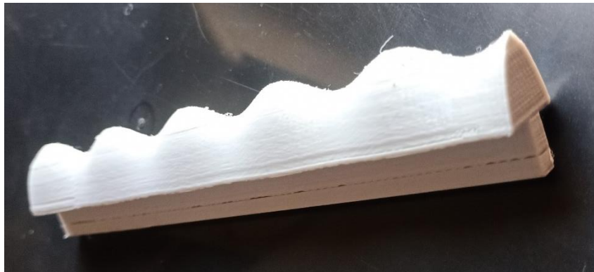
Fig 56. 3D Printed Leading Tubercle
