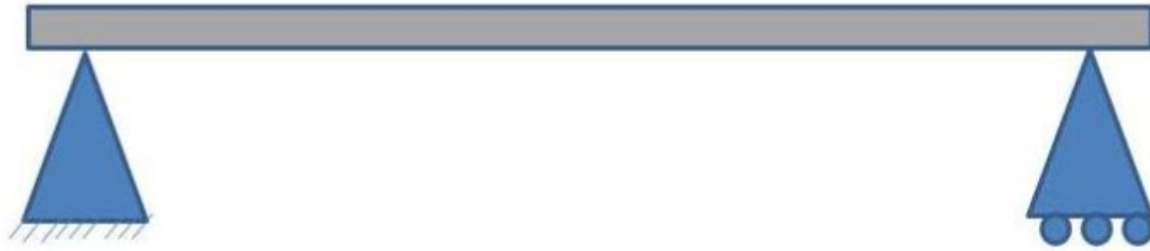
Figure 1: A Simply Supported Beam
