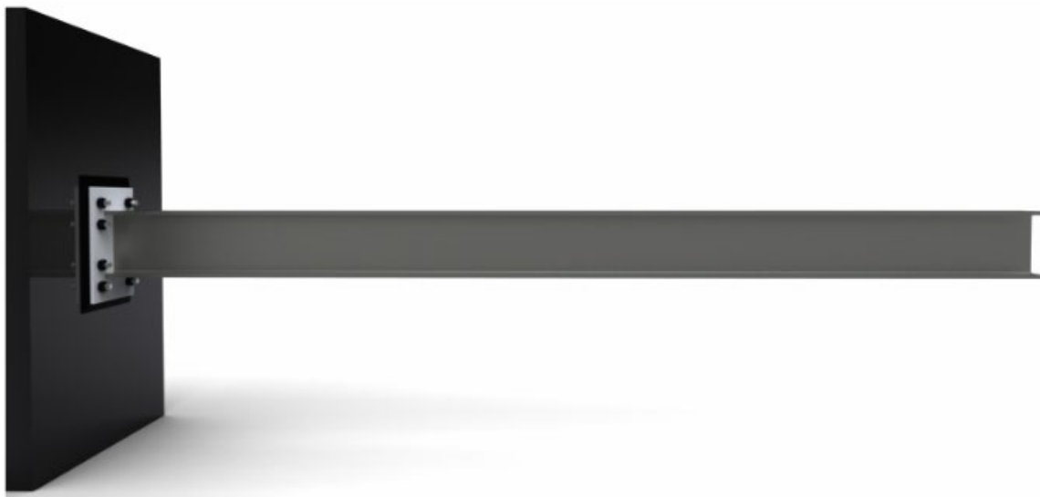
Figure 2: A Cantilever Beam
