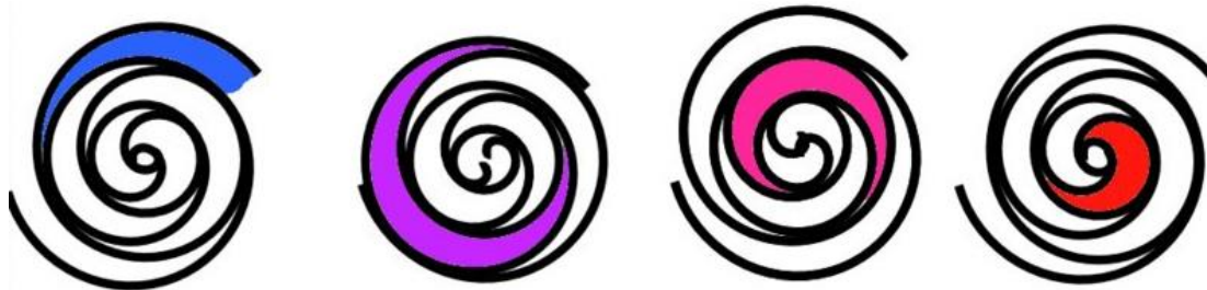
Figure 7: Working principle of the scroll compressor.
