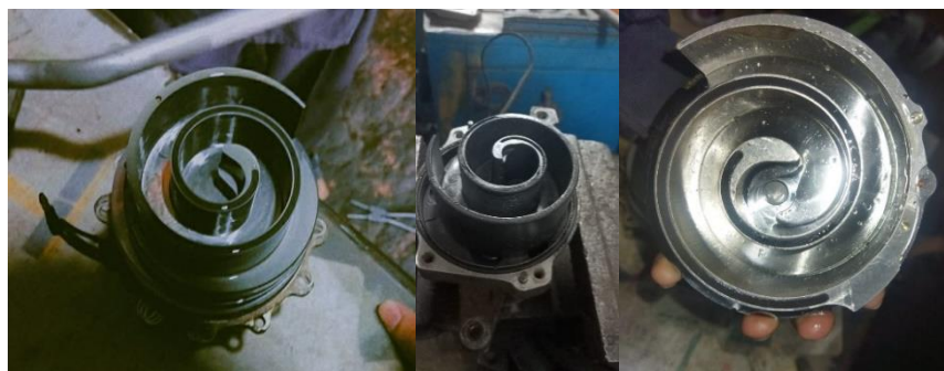
Figure 10: Fix and orbiting scrolls
