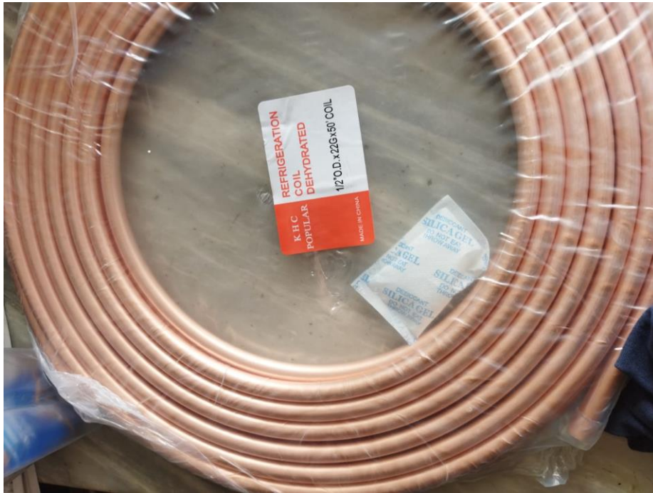
Figure 16: Copper pipe used
