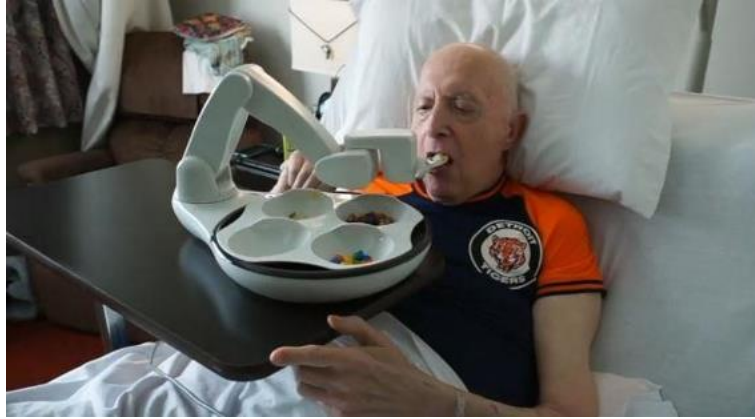
Figure 2. Example of robotic feeding system that is feeding a patient ( www.sciencedirect.com )
