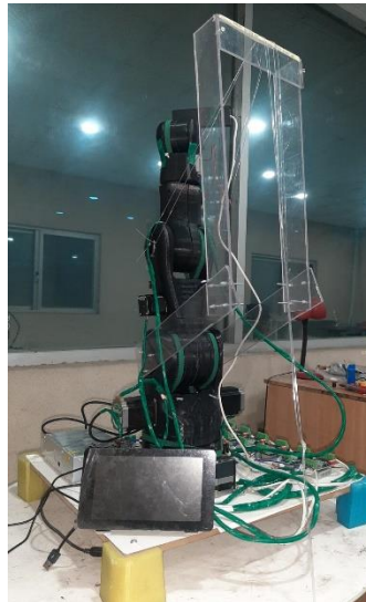
Figure 71: Counterweight assembly with robot
