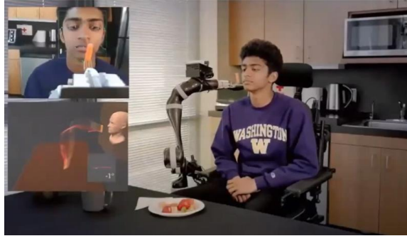
Figure 4. An active feeding robotic manipulator (Source: www.sciencedirect.com/science/article/pii )
