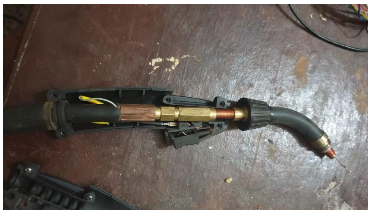
Figure 5 The components within the MIG welding gun
