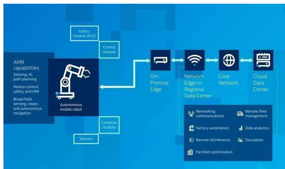
Figure 4 Working diagram of AMR with system components.
