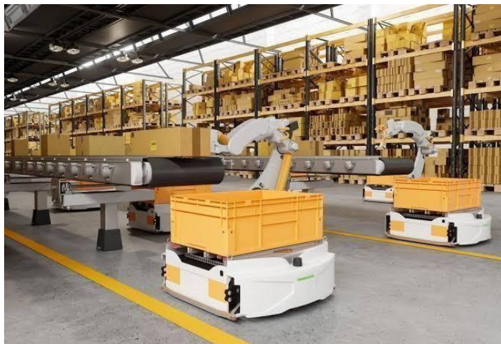
Figure 3 AMRs working in a warehouse to transfer objects from one place to another.
