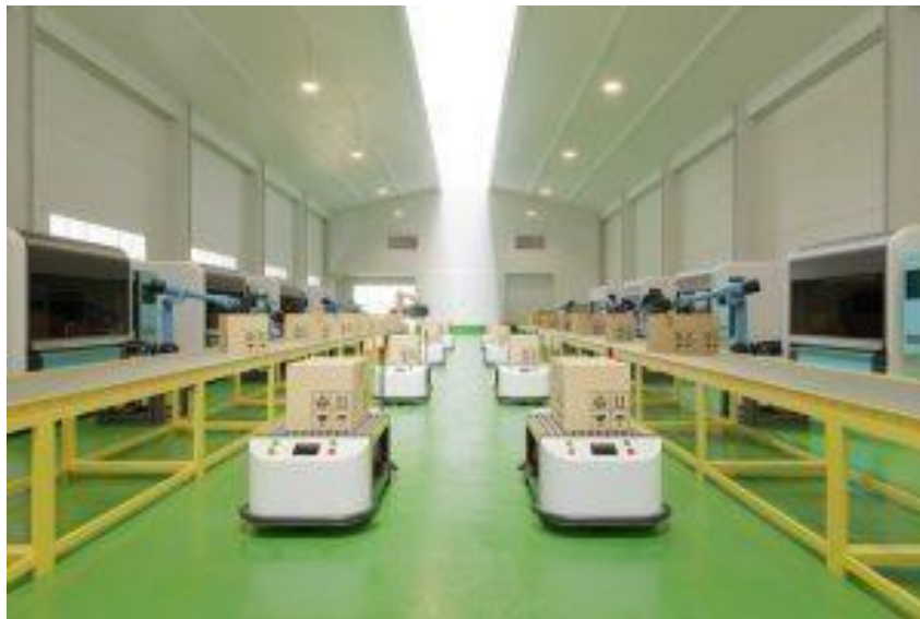
Figure 5 AMRs using LIDAR for path planning and navigation.
