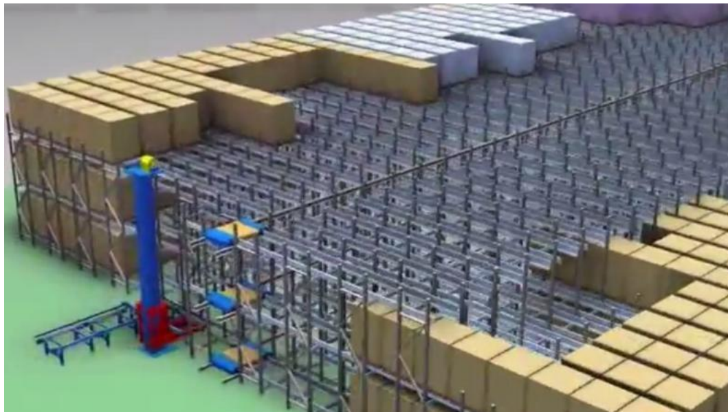
Figure 11 multi-deep compact storage system [17]
