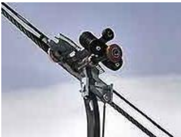
Figure 19 Chair lift self-locking mechanism
