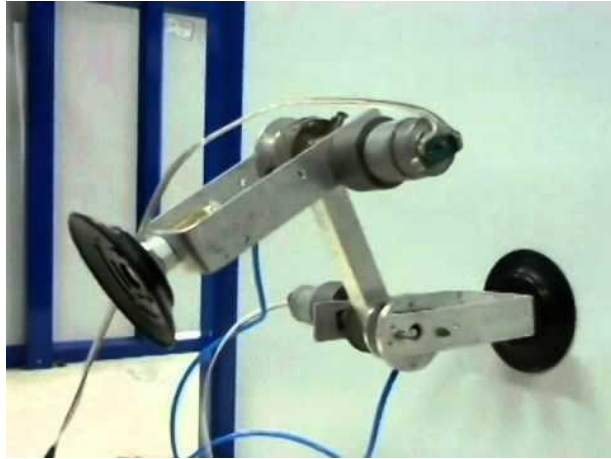
Figure 6: Robot Climbing using suction cups
