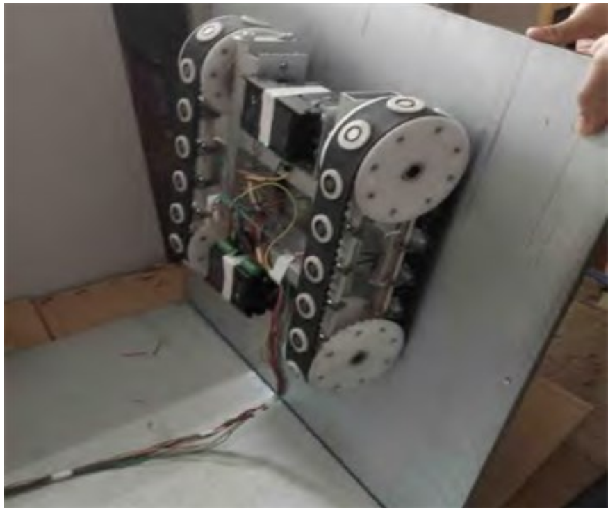
Figure 8: WCR using permanent magnets
