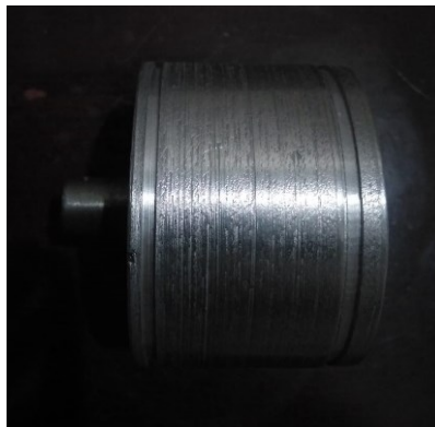
Figure 33: Rim of the wheel; casted with Aluminum
