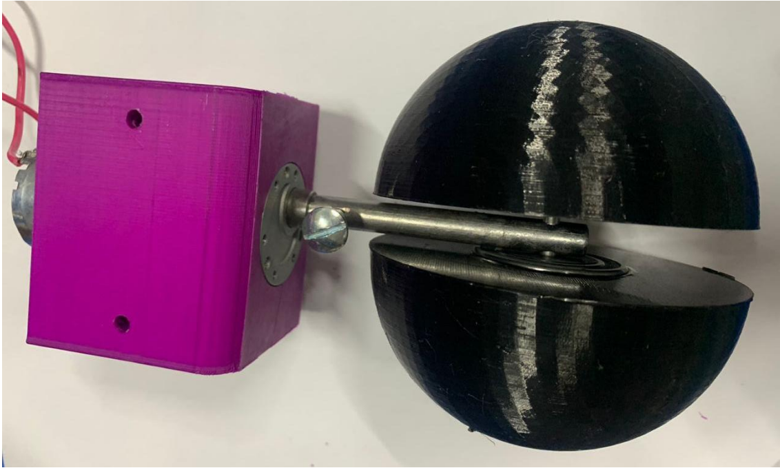
Figure 50. Motor Holder with Motor and Wheel Assembly (Side View)
