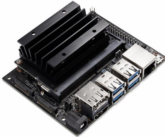
Figure 18. Jetson Nano developer kit. Image courtesy [41]
