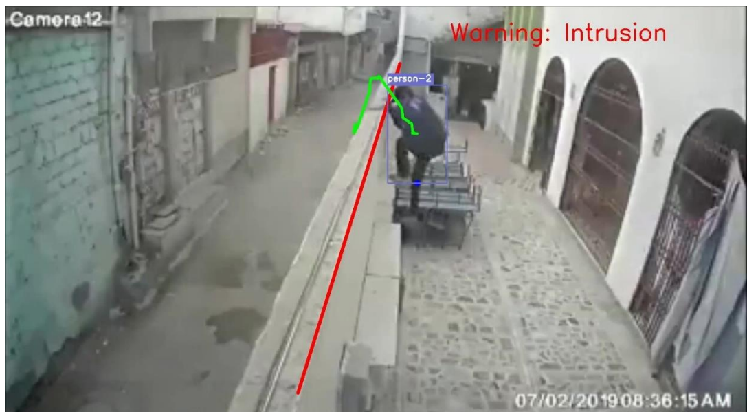
Figure 23. Wall climbing intrusion detection. Image courtesy [43]
