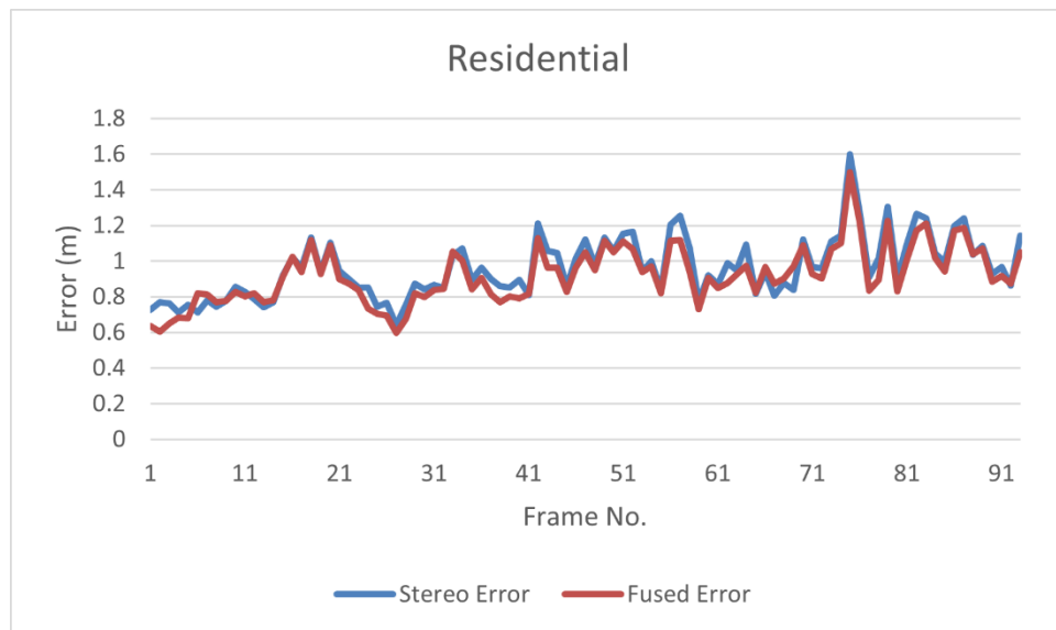
Figure 34. Comparative analysis of errors computed from fused output to the ground truth of a road scene.
