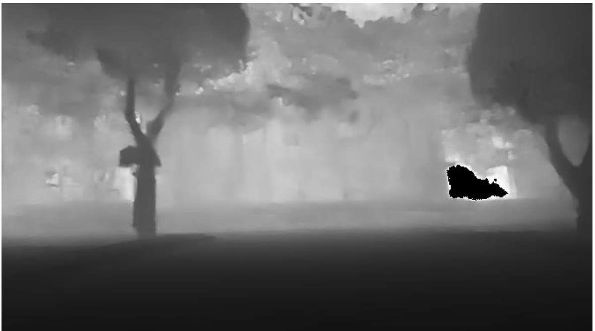
Figure 18. Depth map from stereo camera.
