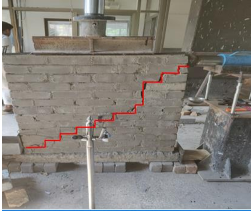
Fig 4.6: Diagonal Stepped Cracking
