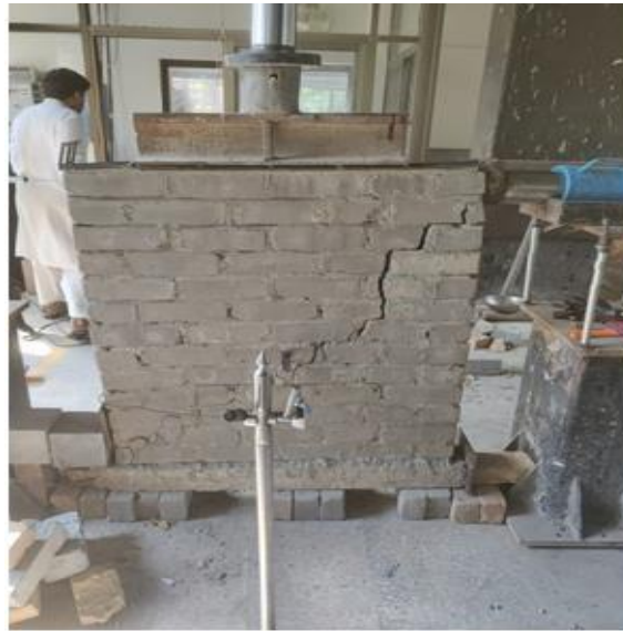
Fig 4.3: Test Result Controlled Fly Ash Wallet
