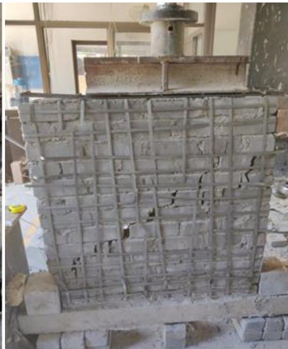
Fig 4.5: Test Result of 100 mm Spaced Retrofitted wallet
