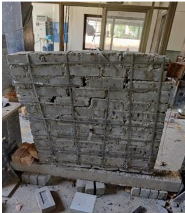
Fig 4.4: Test Result of 200 mm Spaced Retrofitted Wallet
