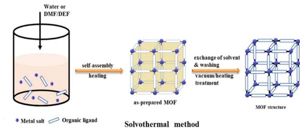
Figure 2.2: Conventional solvothermal synthesis procedure.
