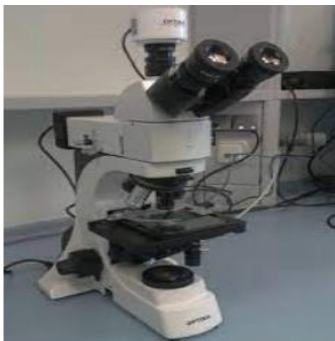
Figure 3.10: Optical Microscope (Optica B-600 MET ) was Used to Analyze the Adsorption of Polymer Chain.
