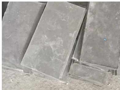
Figure 4: Plastic bricks (20 x 10 cm) made from extrusion process
