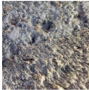
Figure 16: Optical Microscope Image of Plastic Aggregate Showing Surface Texture
