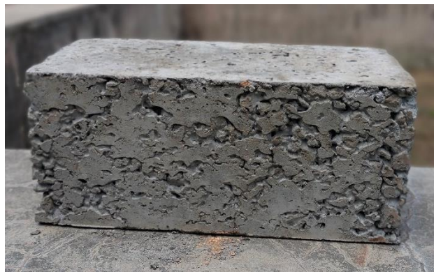
Figure 29: Concrete Block Incorporating Plastic Aggregates
