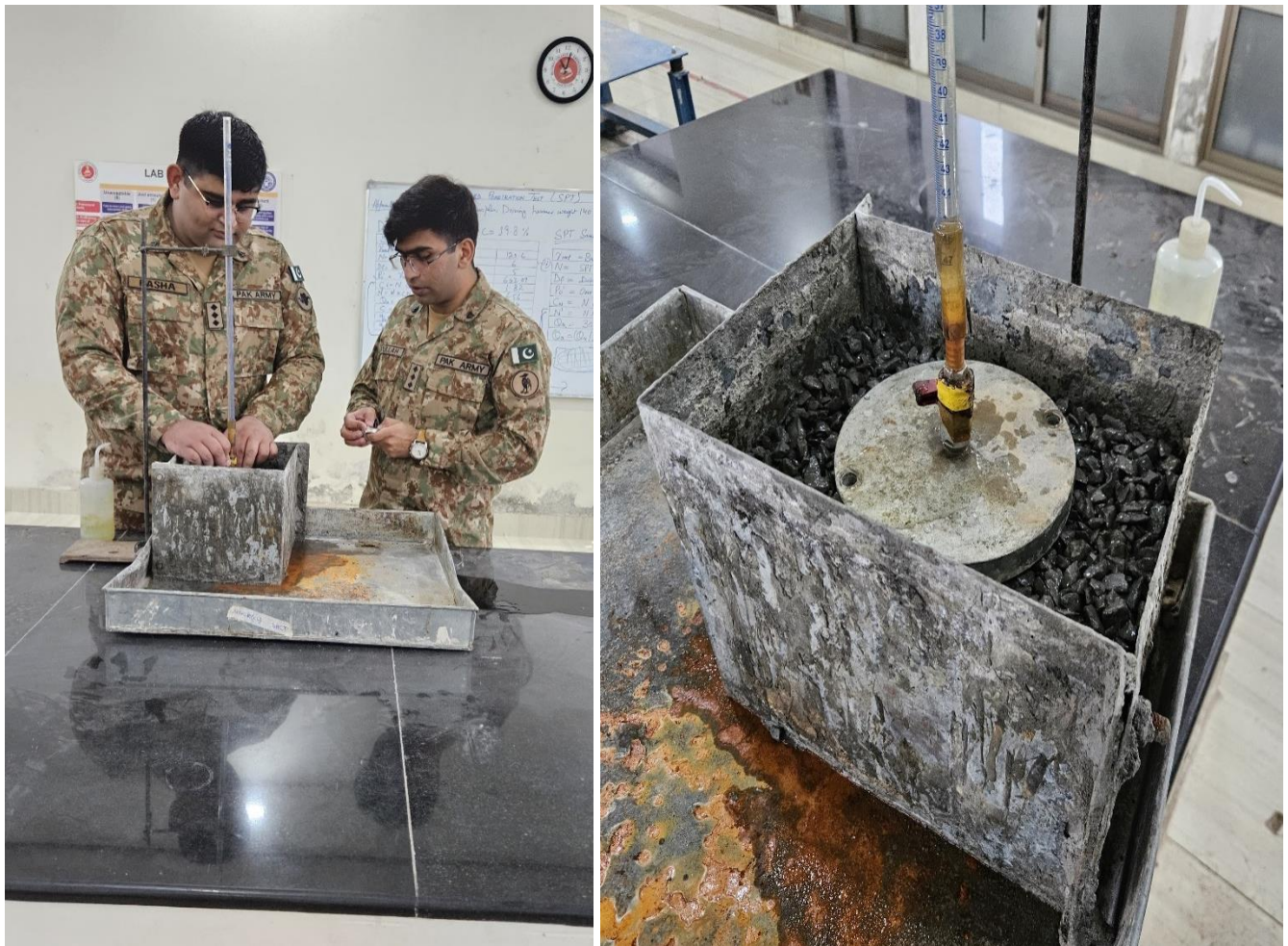
Figure 20: Setting up of apparatus (left). Pervious concrete sample over which apparatus has been placed (right).
