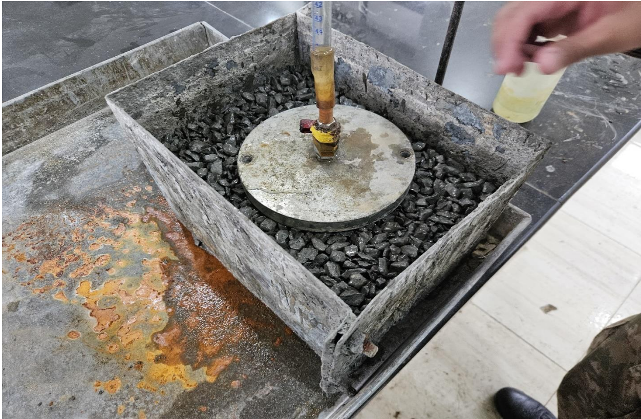
Figure 18: Pervious Concrete Sample (32 cm x 22.5 cm x 25.4 cm)
