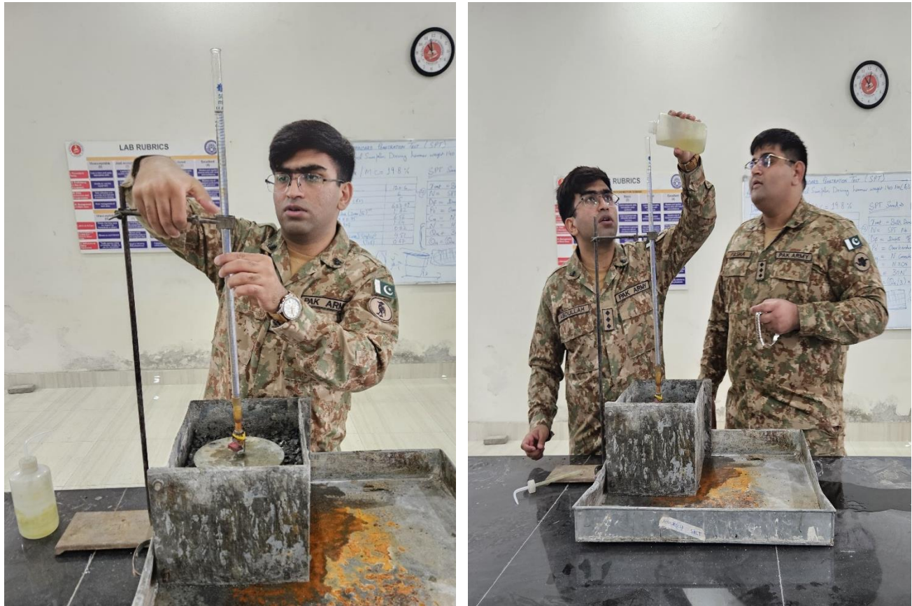
Figure 19: Setting the Falling Head Permeability apparatus (left). Increasing water column height to 35 cm after closing the valve (right)
