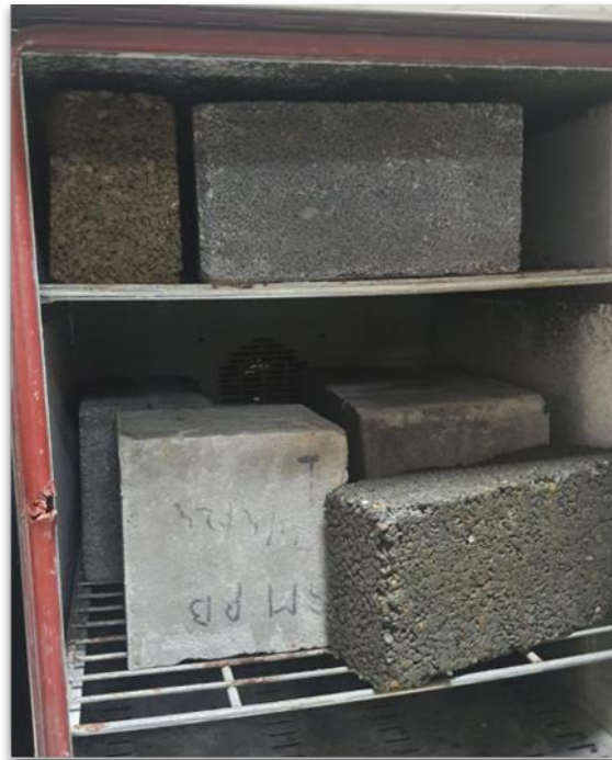
Figure 7: Samples placed in oven for oven dry
