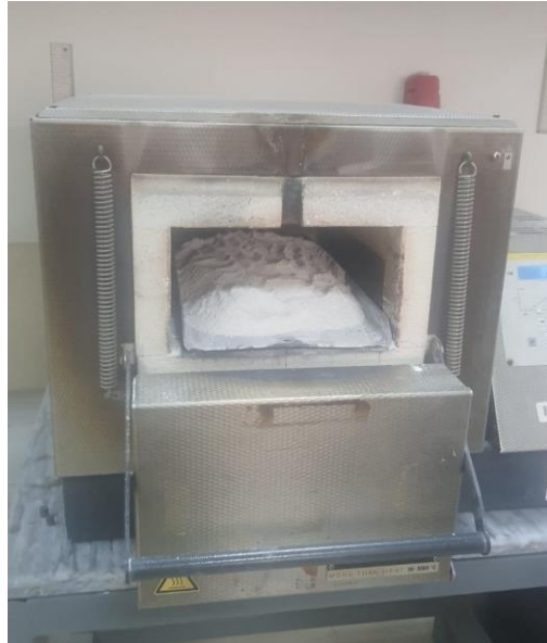
Figure 1: Metakaolin after calcination of kaolin in muffle furnace
