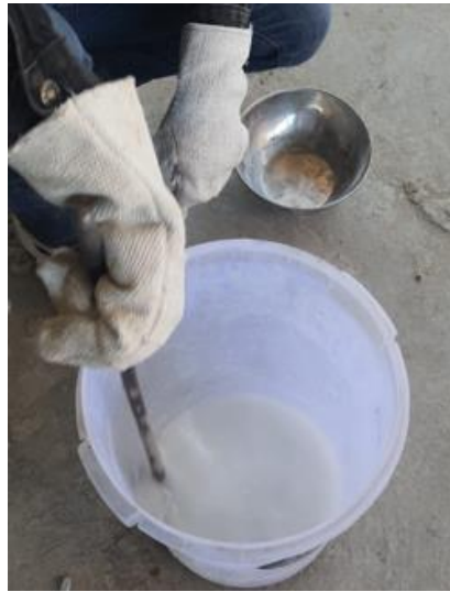
Figure 2: Preparation of alkaline activator solution
