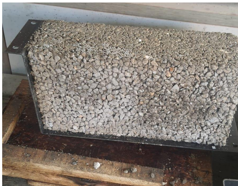
Figure 5: Block sample after demolding for curing
