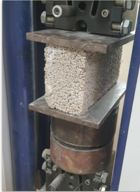
Figure 6: Compressive testing setup
