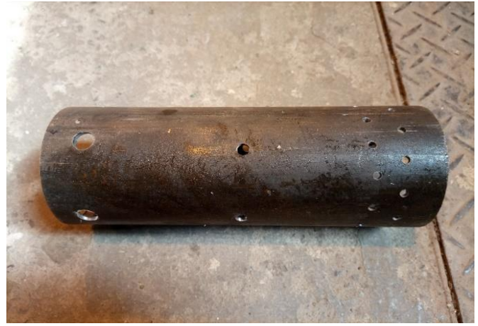
Drilling of holes on combustor liner
