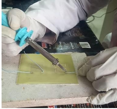
Fig.24. Soldering two wire connection on IDEs.
