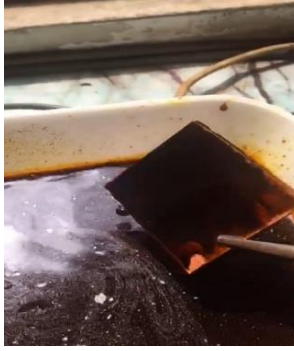
Fig.22. PCB board removed after etching.
