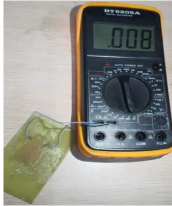
Fig.34. Capacitive sensor after exposure to ammonia.
