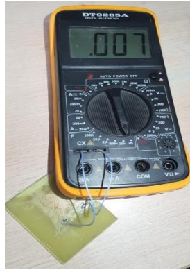
Fig.33. Capacitive sensor before exposure to ammonia
