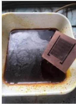
Fig.21. IDE printed PCB board immersed in Ferric Chloride solution.
