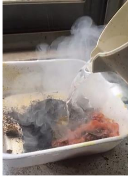
Fig.20. Ferric Chloride being dissolved in water.
