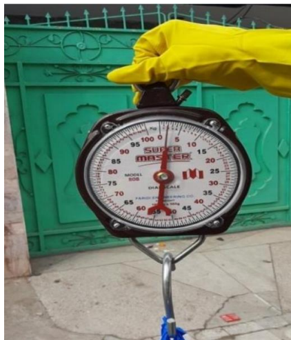
Figure 8: Weighing Machine to Determine Weight of Solid Waste Components
