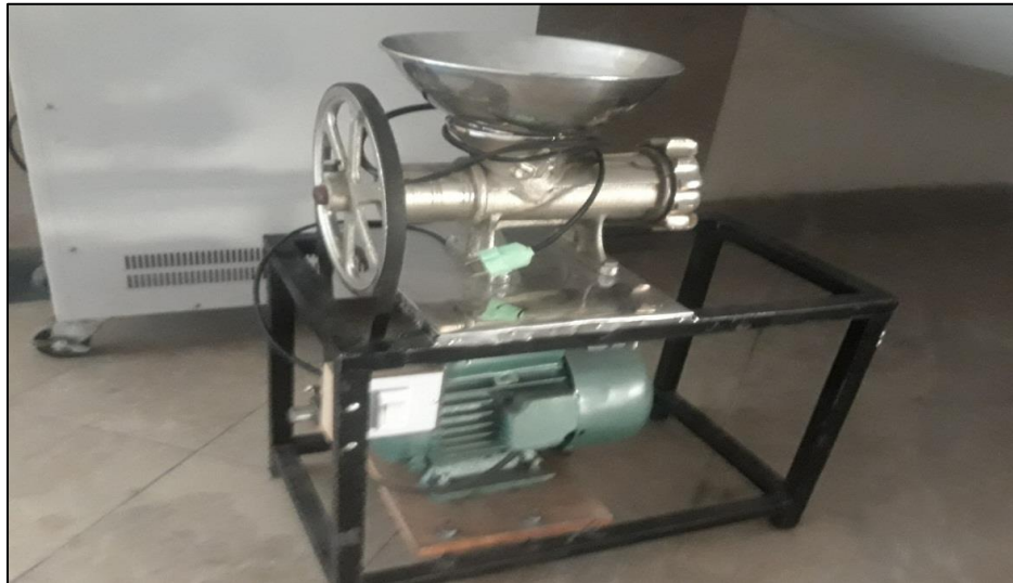
Figure 9: Setup for Shredding
