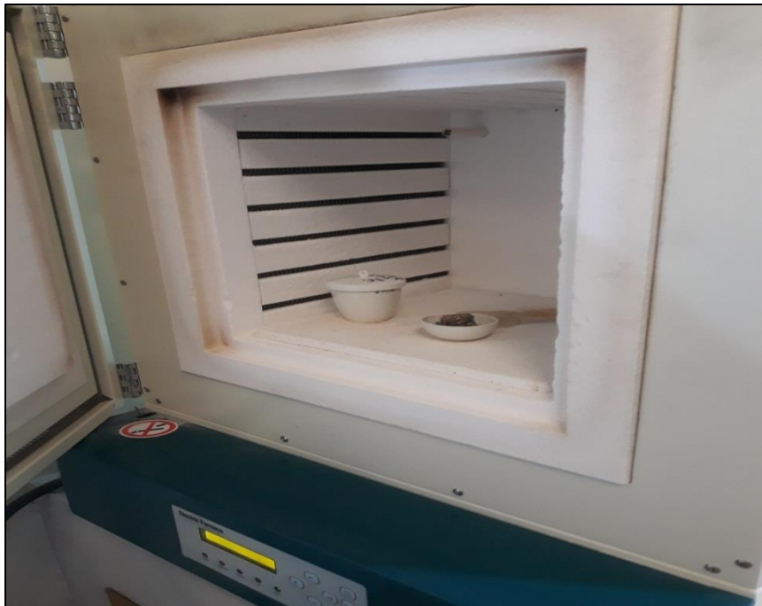
Figure 10: Muffle Furnace used for Proximate Analysis
