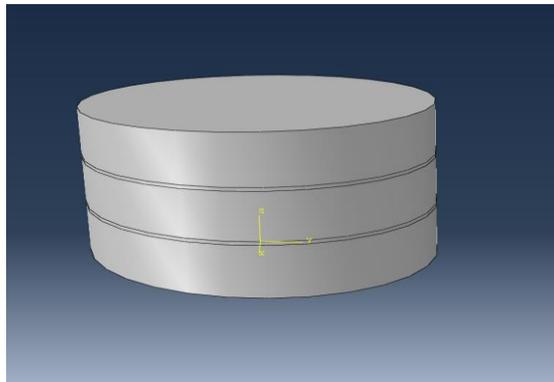
**Figure 15. Piezoelectric harvester formed by connecting three piezoelectric plates.**
