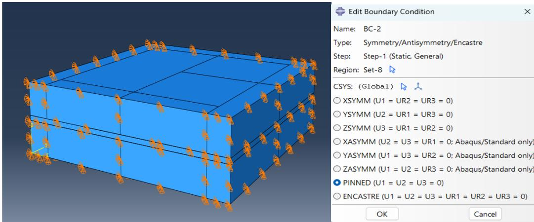
Figure 23. Restraints on bottom and sides (pinned).
