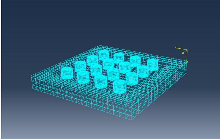
**Figure 18. Mesh of complete PEH in ABAQUS.**
