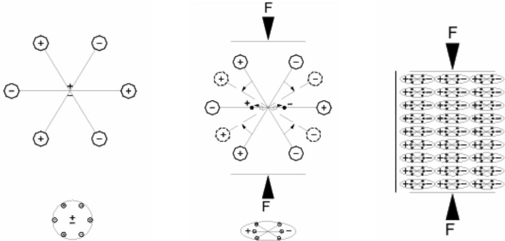
**Figure 1. Left: Normal molecule. Center: Molecule under force. Right: Molecule's surfaces polarized.**
