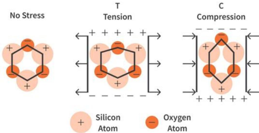
**Figure 5. Atomic structure of a Piezoelectric.**
