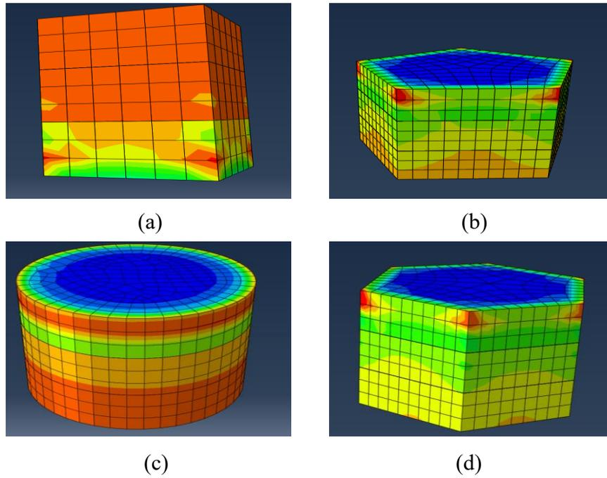
**Figure 25. Sections used for PZT disks; (a) Square, (b) Pentagon, (c) Circular, (d) Octagonal.**
