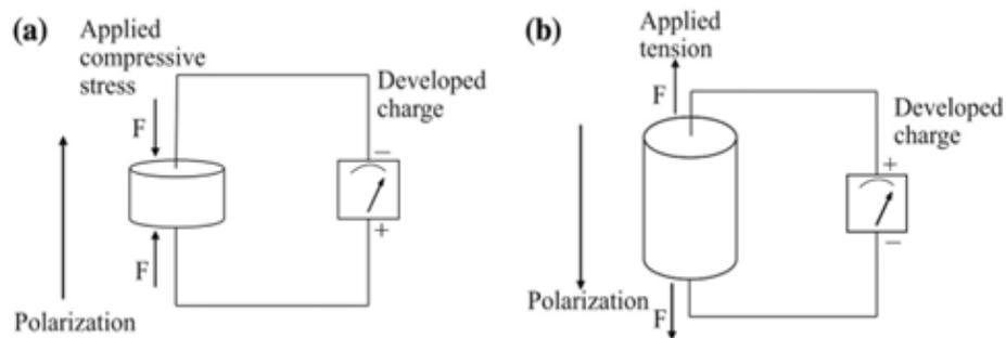
**Figure 2. Relation of direction of force with polarization.**
