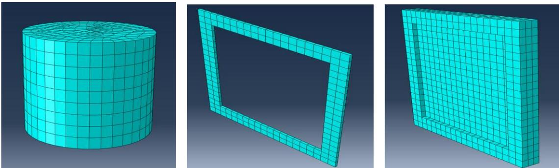
**Figure 19. Mesh of Piezoelectric harvester (left), Rubber seal (middle), MC Nylon casing (right).**
