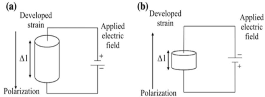
**Figure 3. Relation of strain developed with polarization.**
