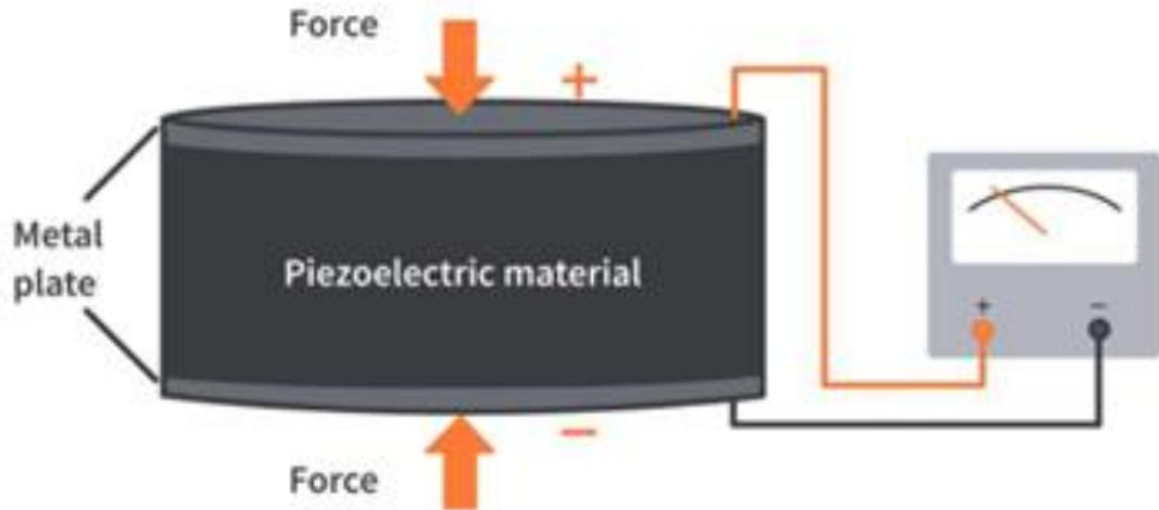
**Figure 6. Working principle of piezoelectrics.**
