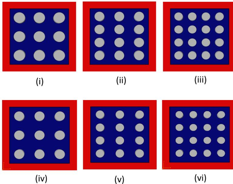
**Figure 16. PZT disks distributions in PEH by: (i)  $3 \times 3$  (dia = 2.3 cm), (ii)  $3 \times 4$  (dia = 2 cm), (iii)  $4 \times 4$  (dia = 1.73 cm); (iv)  $3 \times 3$  (dia = 2 cm), (v)  $3 \times 4$  (dia = 1.73 cm), (vi)  $4 \times 4$  (dia = 1.73 cm). Total area Piezoelectrics (above) = 37.7 cm<sup>2</sup>; Total area Piezoelectrics (below) = 28.27 cm<sup>2</sup>.**
