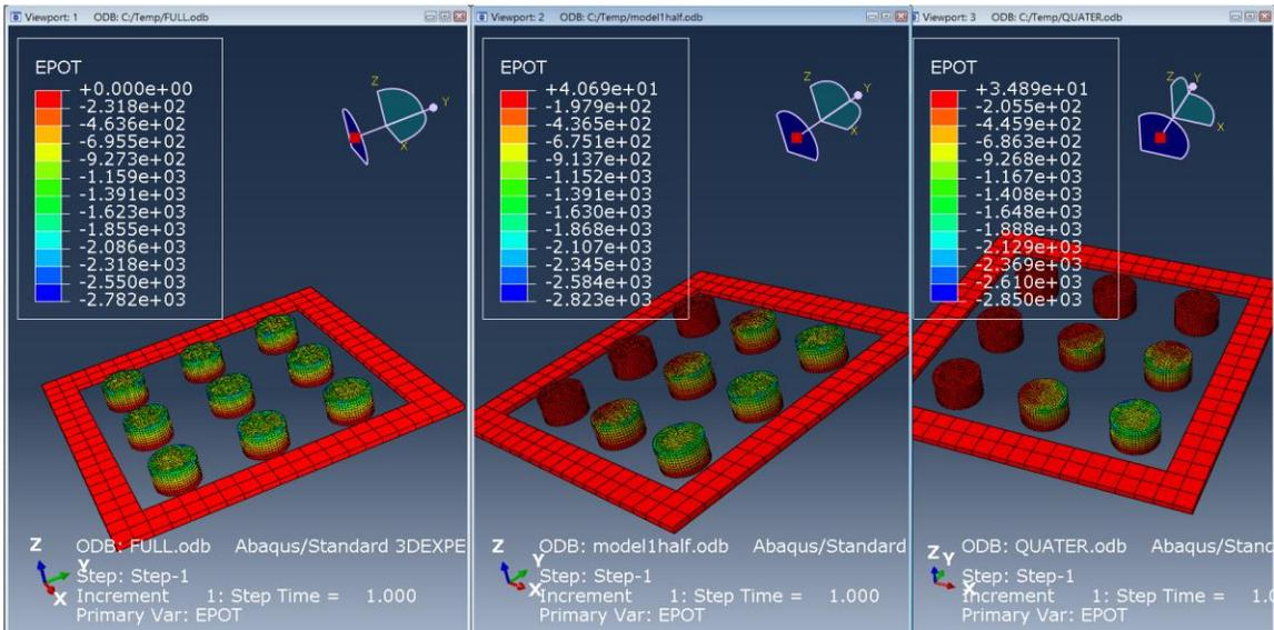
**Figure 22. Electric Potentials are obtained through three different loading conditions. Full (left), Half (middle), Quarter (right).**
