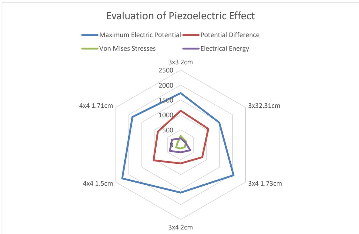
**Figure 30. Outputs of different PEHs plotted on a Radar Chart.**
