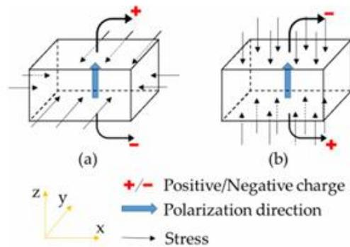
**Figure 10. Modes of operation for PZT materials: (left) 3-1; (right) 3-3**
