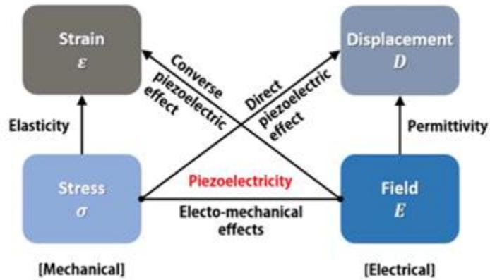
**Figure 7. Different piezoelectric effects.**
