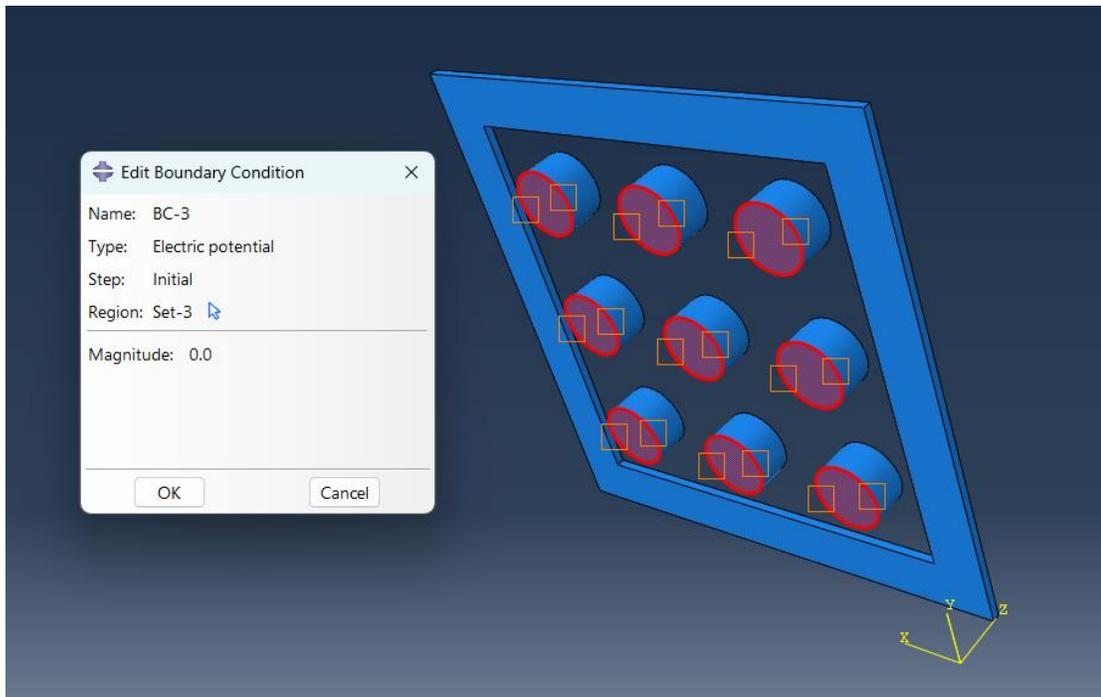
Figure 24. Setting Boundary conditions in ABAQUS software.
