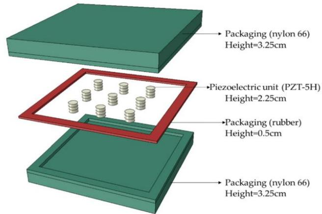
**Figure 14. Overview of PEH finite element model. (Cong Du, et al. 2021).**
