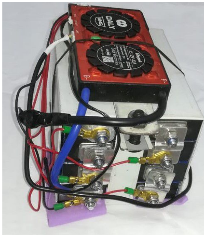
Figure 3.1: LiFePO 4 batteries with BMS
