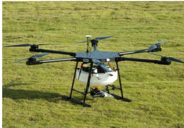
Figure 4 A sample hexacopter drone with pesticide sprayer
