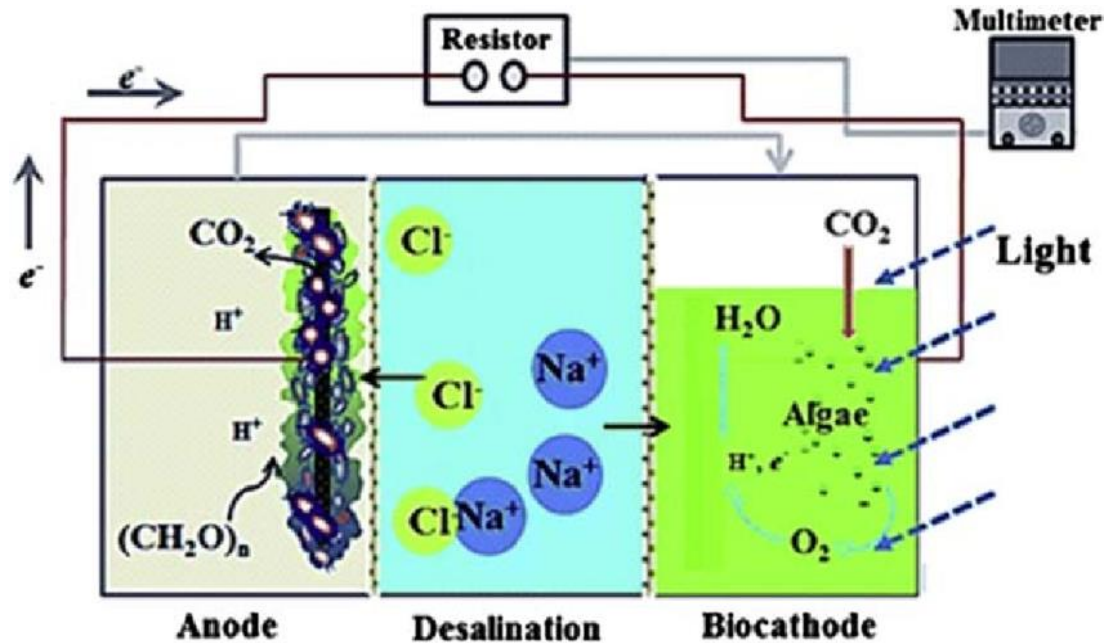
Figure 2.2 Photosynthetic Microbial Desalination Cell (PMDC), source: (Kokabian & Gude, 2019).
