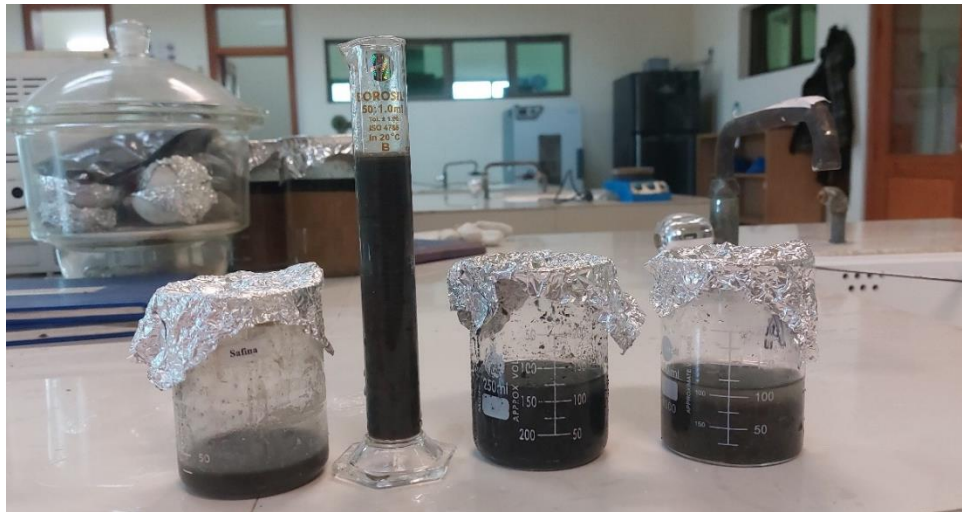
Figure 3.3 Anaerobic Sludge inoculation in anode chamber.
