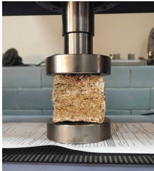
Figure 12 - Compressive Strength Test on Uncompressed samples
