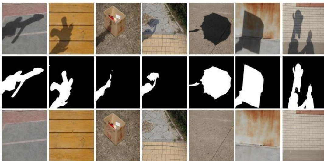
Figure 3.3: Examples of samples added in training dataset from shadow and shadow-free Pair Images by generating the shadow-mask
