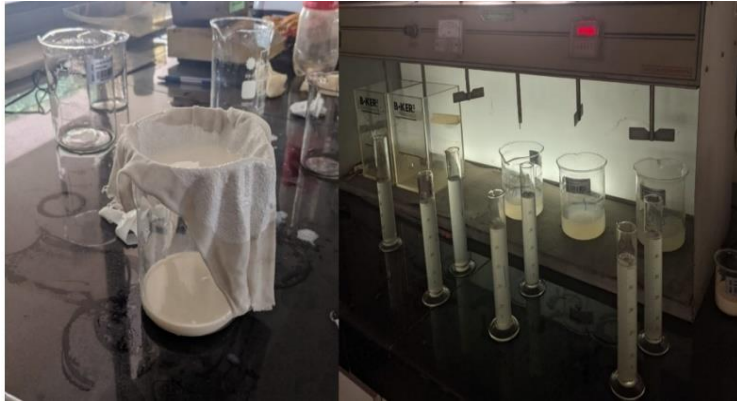
Figure 19. Coagulant Filtration Process
