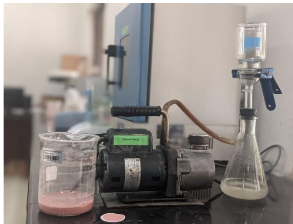
Figure 5. Lab apparatus for measuring TSS
