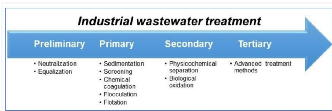
Figure 1. The process chain of Industrial Wastewater Treatment
