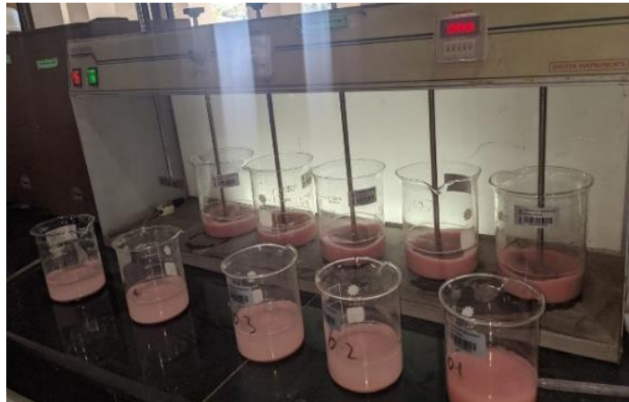
Figure 21. Settling of TSS in PIW after coagulation
