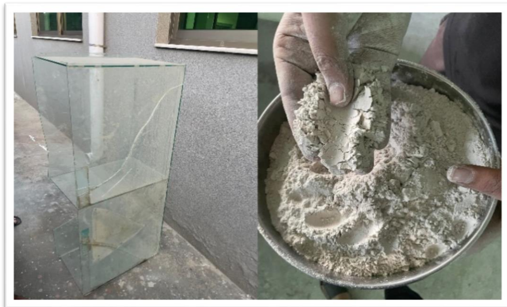
Figure 2 Waste glass crushed into powder form
