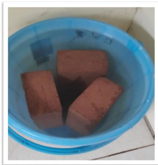
Figure 15 sample bricks placed in water tub
