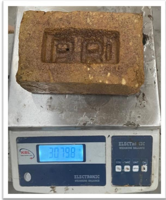
Figure 17 Weighing wet brick sample
