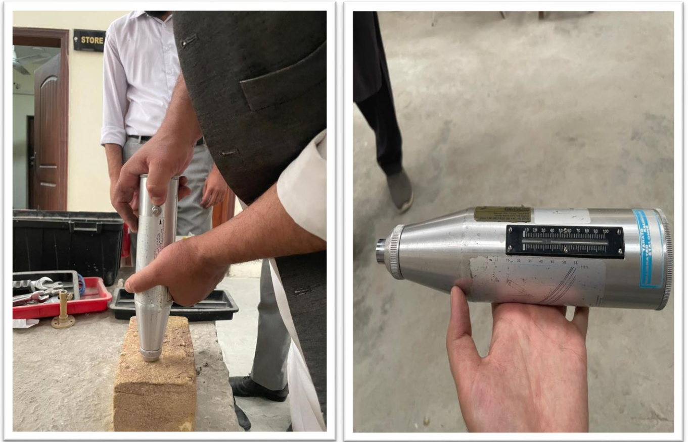
Figure 14 Figure 14 Performing Rebound Hammer test at MCE Structural Lab
