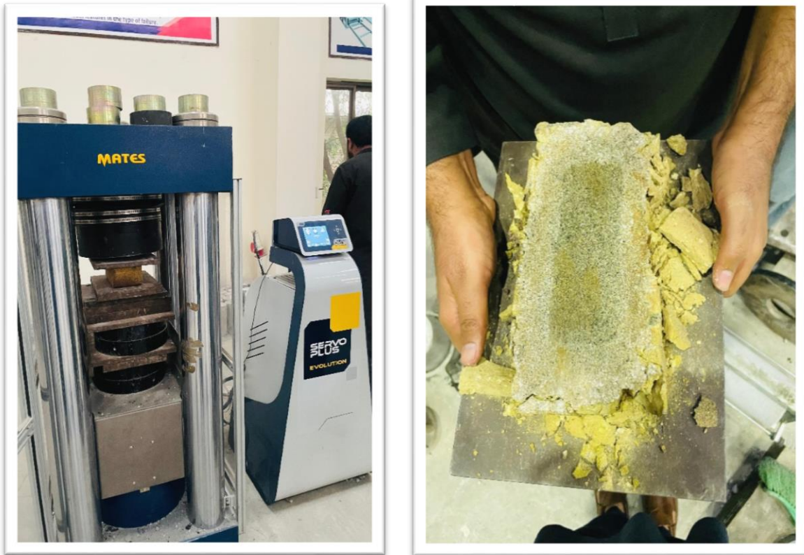
Figure 10 Performing compressive test on brick samples
