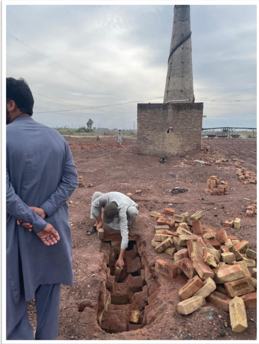
Figure 5 Baked bricks being extracted from Kiln
