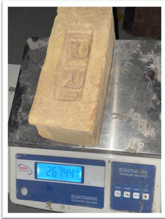
Figure 16 Weighing dry brick sample
