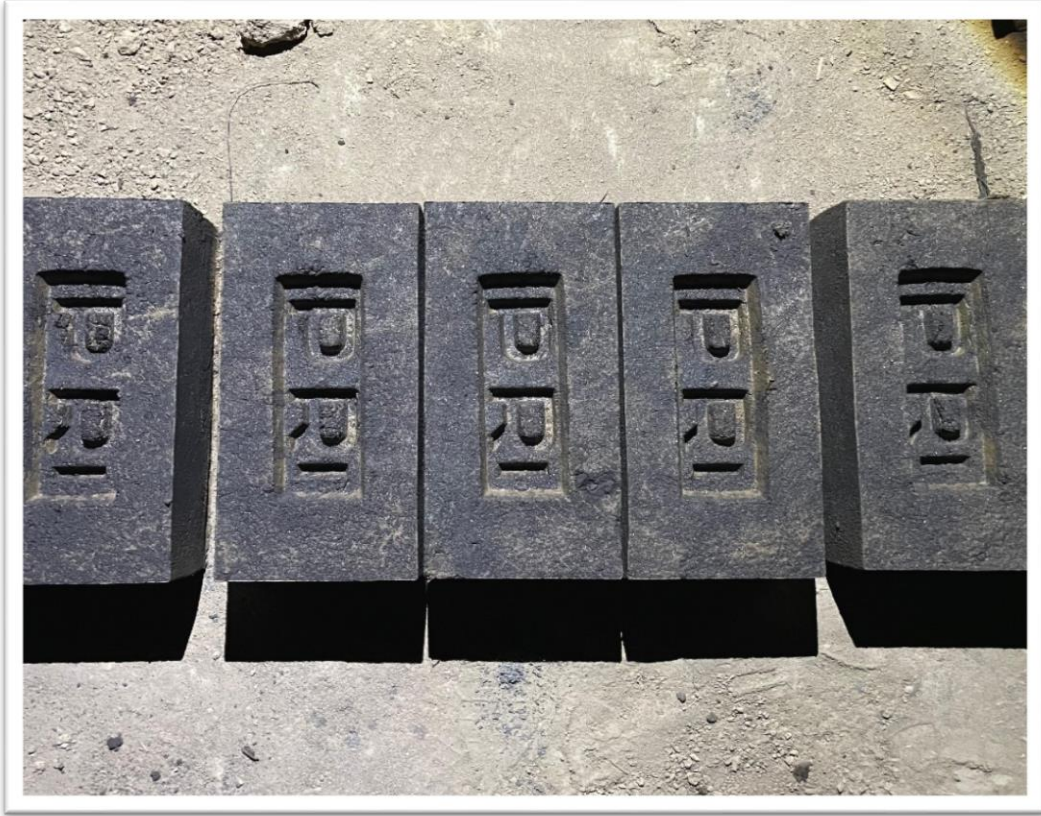
Figure 4 Prepared Brick samples before baking
